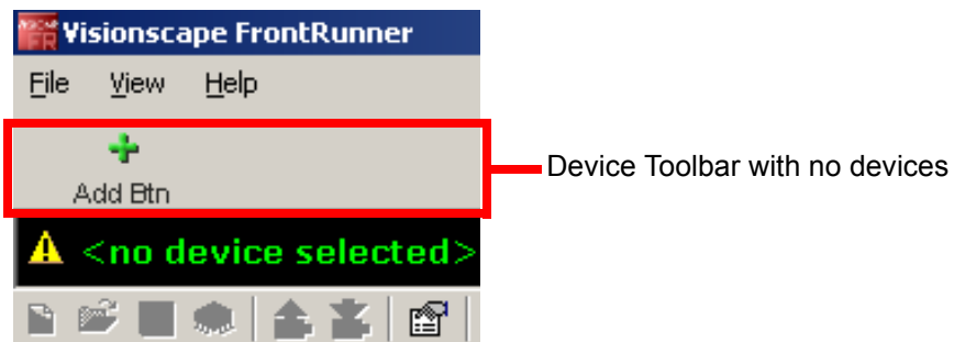
FIGURE 2-2. Initial FrontRunner Startup - No GigE Cameras or Software Systems
